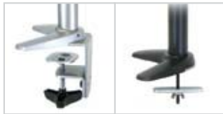
Clamp and grommet bases included: clamp to surfaces 1/2–1 7/8" (13–48 mm) thick or grommet mount through holes 5/16–2" (8–51 mm) wide, up to 2 1/2" (63 mm) thick
