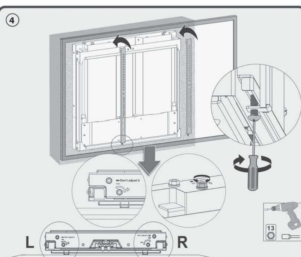
The mount arrives with a default balance setting. Two balance bolts (one located on each side-left and right) must be adjusted to set proper balance using a drill as shown. Adjust the bolts clockwise/counter-clockwise (5 sec recommended for each action), alternating between each side until it has achieved a perfect balance.
