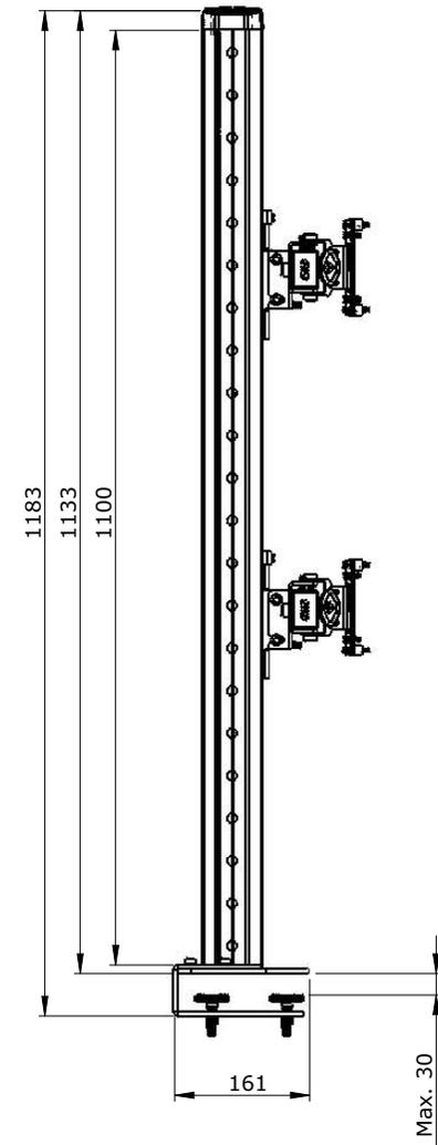
MM051012-P0 SMS Multi Control 2xDual Boomerang dimensions in mm
