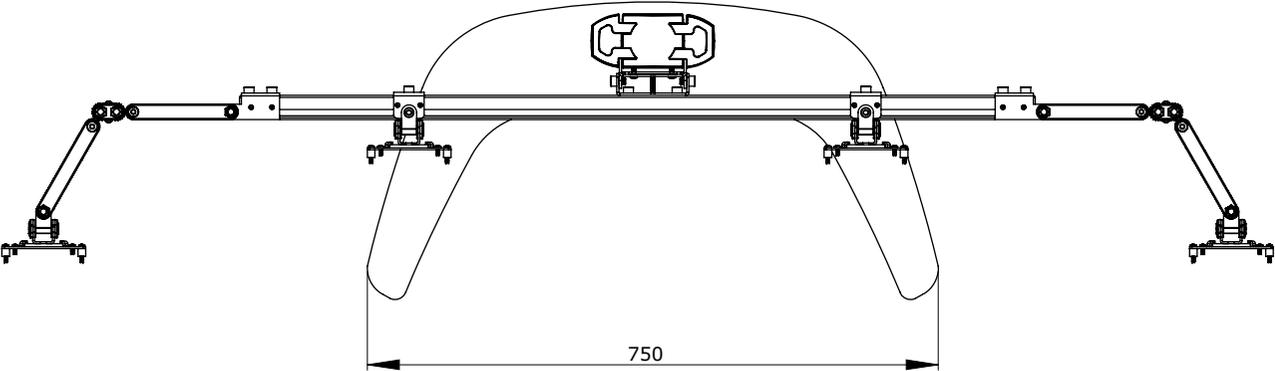
MM051011-P0 SMS Multi Control 2xDual Clamp dimensions in mm
