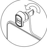
Secure the key, push the cam lock inwards and rotate 180° anti-clockwise until it clicks
