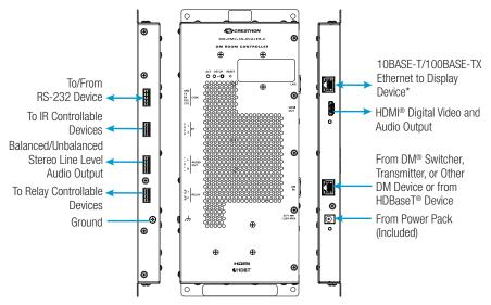
\*Do not connect the LAN port to an Ethernet switch if the DM IN port connects to a DM switcher. If the DM IN port does not connect to a DM switcher, the LAN port can connect to an Ethernet switch.
