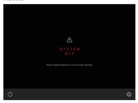
Tap the (gear) icon to the right of the (power) button to display the **System**Configuration screen. If the gear icon is not visible on the main screen, touch and hold the bottom right corner of the screen for 10 seconds to display the **System Configuration** screen.
