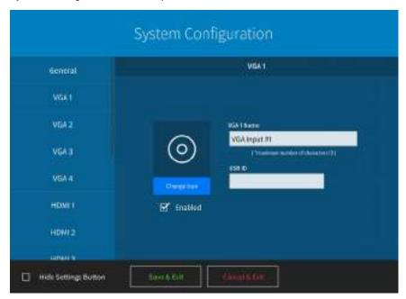
Use the **Name** text box to enter the input name you want to display on the source selection screen (shown on page 22).
