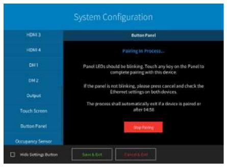
5. Push any button on the MP-B10 to complete the process. The screen will indicate the .AV Framework host device is paired with the MP-B10.
