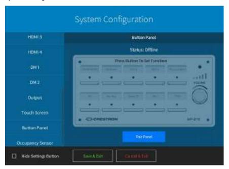
3. Tap Pair Panel to access the button panel configuration controls.
