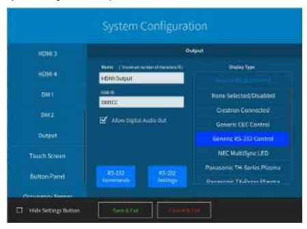
Use the Name text box to enter the output name you want to display on the main screen.
