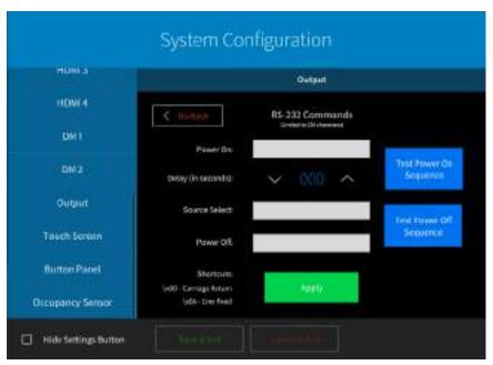
Tap Go Back to return to the Output screen, and then tap RS-232 Settings to display the settings configuration screen
