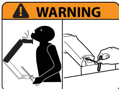
**WARNING! Stored Energy Hazard:** The arm mechanism is under tension and will move up rapidly, on its own, as soon as attached equipment is removed. For this reason, DO NOT remove equipment unless the arm has been moved to the highest position! Failure to follow this instruction may result in serious personal injury and/or equipment damage!
