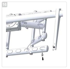
Power and signal cables may be conveniently run through the arms of the mount between the display and the power and signal source to assist in the clean look of the cable installed.
