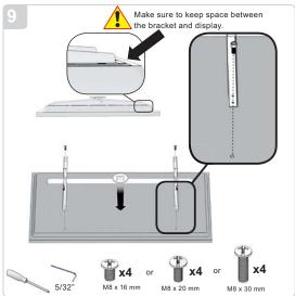
Invert the flat panel display and place it on a smooth flat surface so the back of the display panel is facing up. Align the two mounting bracket to the four mounting points on the rear of the display and secure them bracket to the display with the proper "pitch" supplied hardware. Check the owners manual to determine correct pitch hardware recommended.
