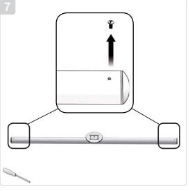
Remove the two security screws from the right and left side of the mounting bracket crossbar and slide the two mounting brackets inside the left and right side security screw hole and reinstall the two security screws.
