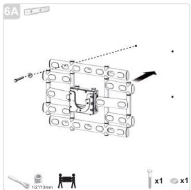
With minimum two people place the PFW6856 wall plate assembly and secure to the wall using the top center hole of the wall plate.
