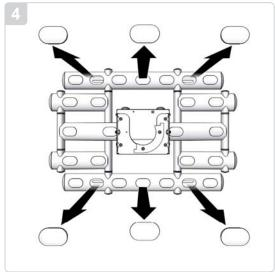
Take the mounting template supplied insure the template is centered and level at the desired height on the mounting surface. Mark the mounting hole (six recommended) three on top and three on bottom.
