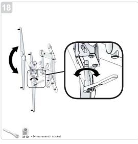
The PFW6856 has a unique "load offset adjustment" feature that allow for the heavier weight displays to be tilt corrected past base center back to level from top to bottom. With personal lifting gently "out " on the bottom of the display a 9/16" (14mm) socket may be used to increase or decrease the tilt feature of the mount.
