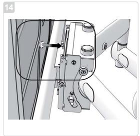
With the cross bar fully seating into the receiver reinstall the (6mm) safety knurl knob.
